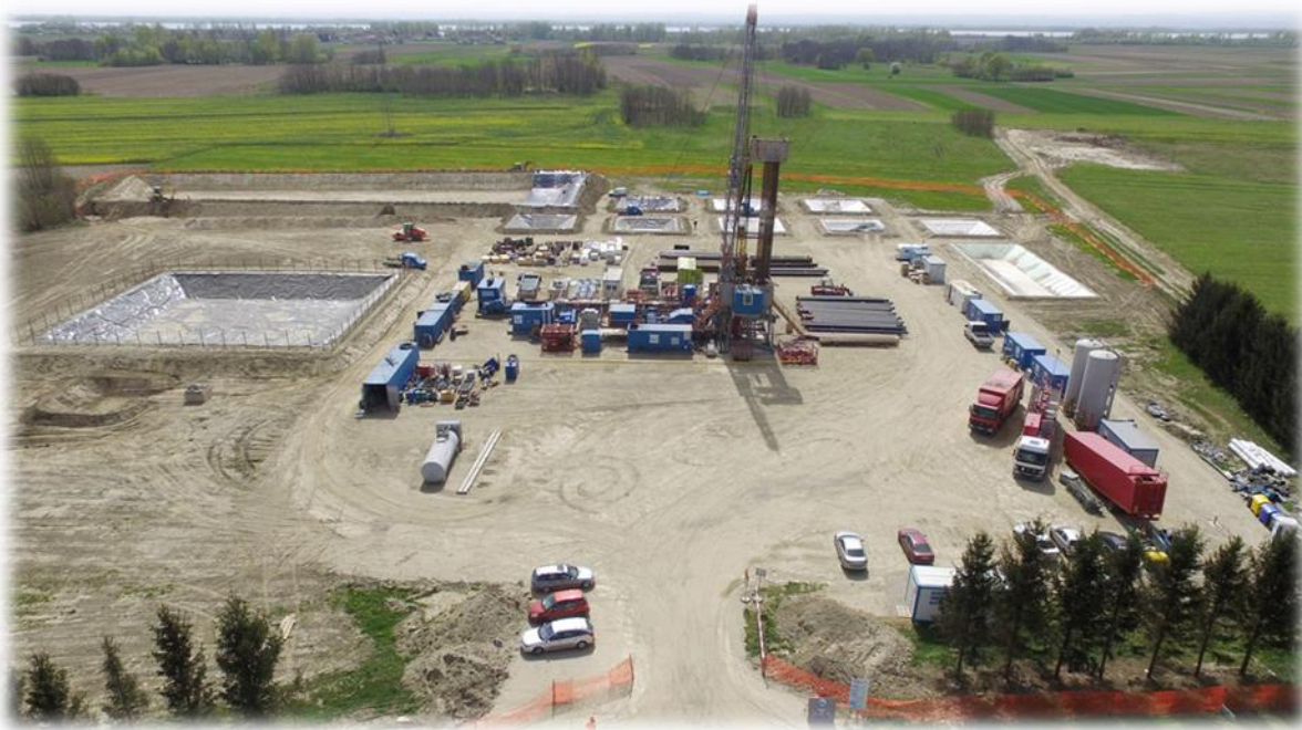
Picture1.4An example of the appearance of the borehole working area of an exploratory geothermal well (Source: EZO-Draškovec)
