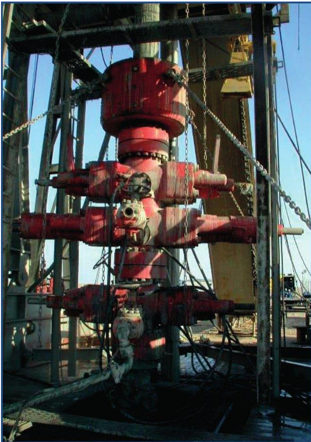
Picture1.13 Example of a typical preventer assembly (BOP) (Potter, 2018)
