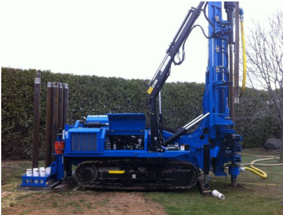
Picture1.6 Geo-Max drilling rig for making geothermal wells (Source: https://drillingsupply.info/geothermal-drilling-rigs/geothermal-drilling-track-rig-gm840-dd.html )
